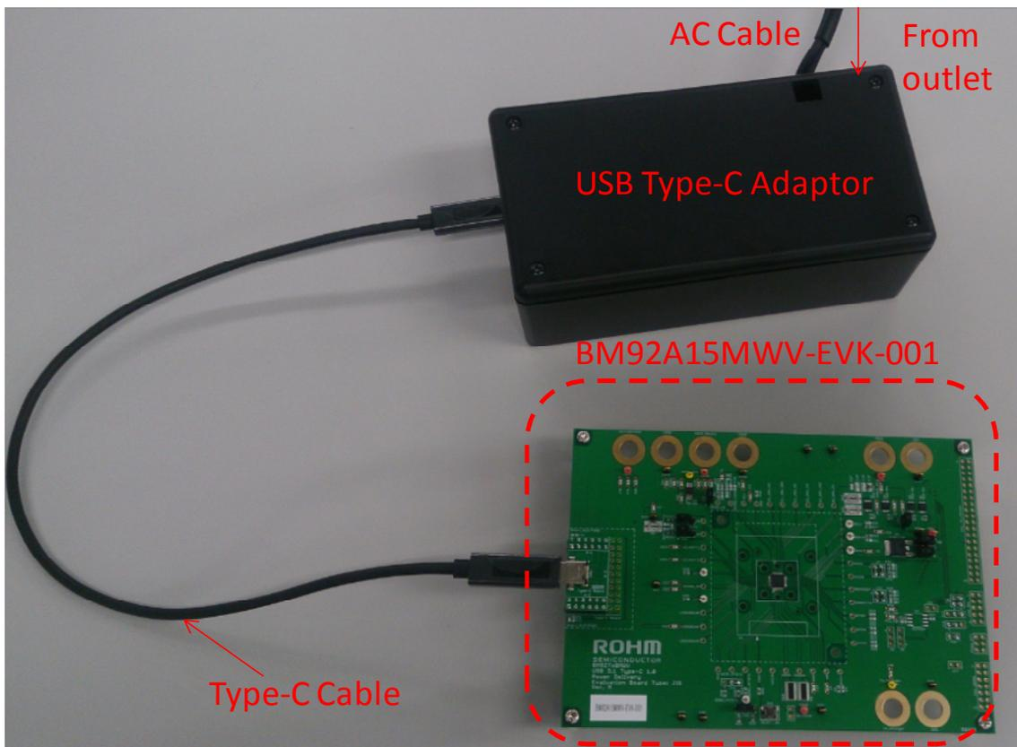
Figure4. Device connection photo using Type-C cable
